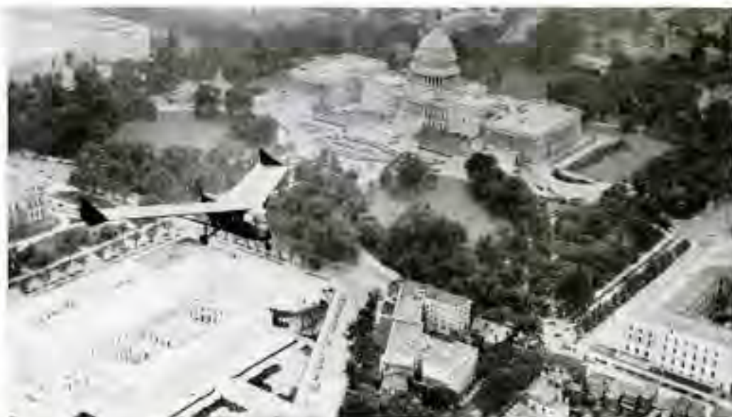
The Waterman plane flying over Washington, D. C. This photo clearly shows the wing arrangement and the controls mounted on the wing tips.
