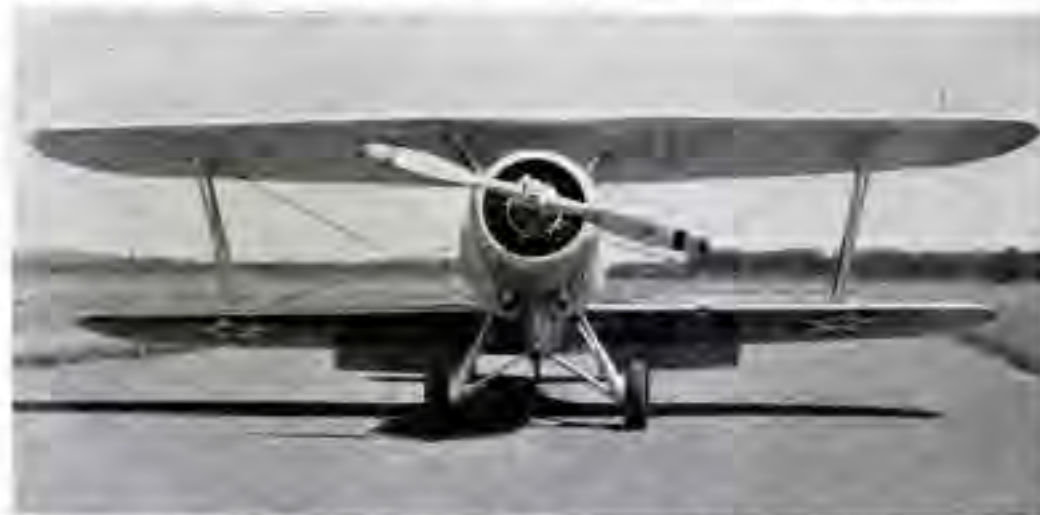
Front elevation of the Vought SBU-1 Scout-Bomber showing the trailing edge flaps depressed.
