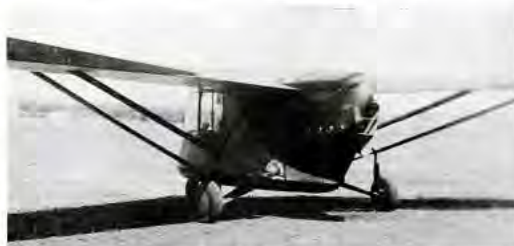
A rear view of the Waterman plane showing the engine cowling and landing gear arrangement.
